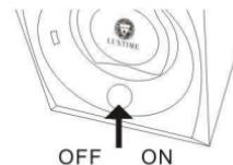
When the switch is pushed to the on position, the color indicator in the switch will light up in red and green at the same time for several seconds, which indicates the device is being initialized.
